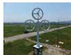
9 kW multi-lens wind turbine (Kitakyushu City Chuki is experimenting to obtain certification) Certification is scheduled to be acquired in March 30 (grid connection)
