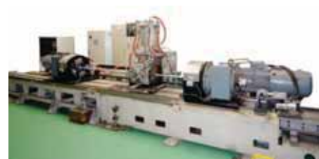
Examples of RMACREO devices: (Diameter 50 mm×4000 mm can be processed)
