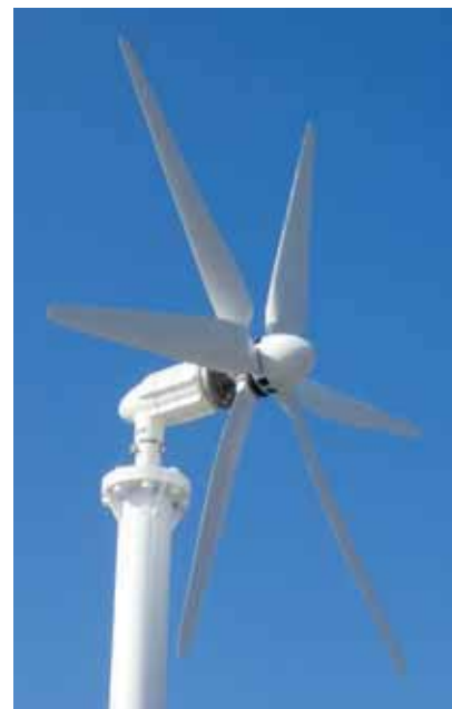
1 kW (2.2 m diameter) wind turbine currently in operation in Higashi-ku, Fukuoka-shi and Kurume-shi
