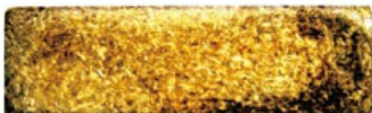
(A) Specimen of woodchips 100% with adhesive (Woodchips size: 1mm or less)
