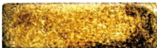
(A) Specimen of woodchips 100% with adhesive (Woodchips size: 1mm or less)
